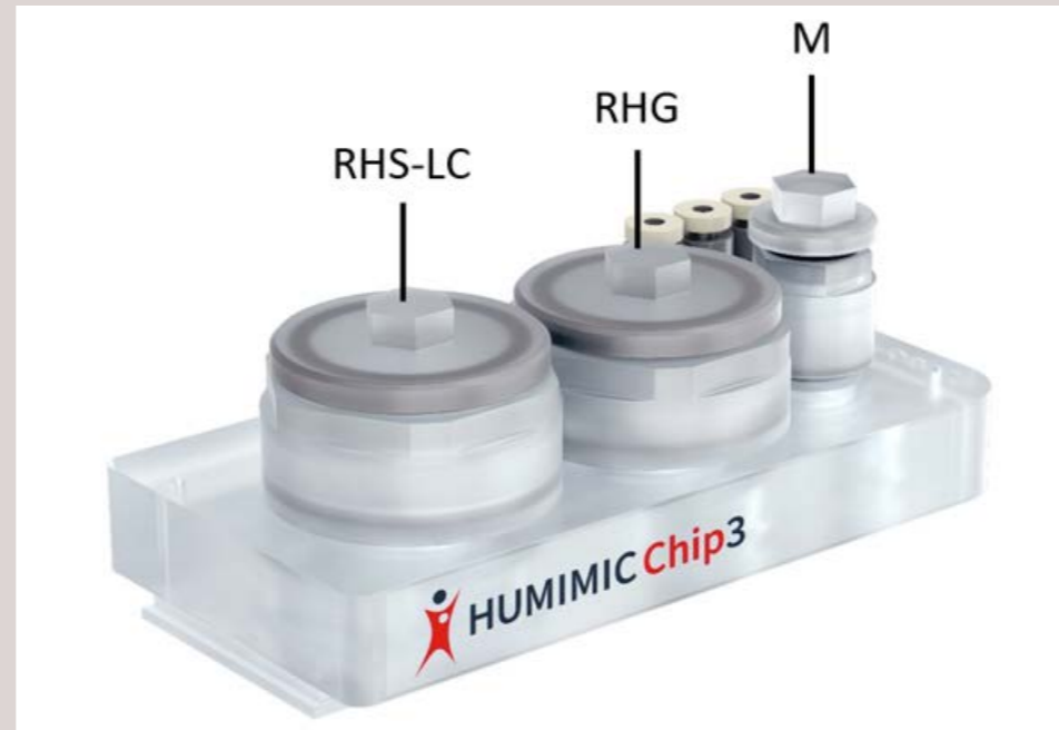
Figure 1: experimental overview of HUMIMIC multi-organ Chip with reconstructed human gingiva (RHG) and reconstructed human skin with Langerhans cells (RHS-LC). M = medium reservoir
