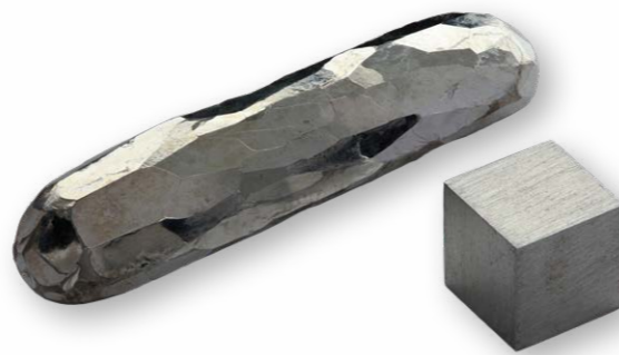
Afb. 1. A crystal cadmium bar. Purity 99.999 %. Made by the flux process. As well as a 1 cm 3 cadmium cube for comparison. By: Alchemist-hp (talk) (www.pse-mendelejew.de)
